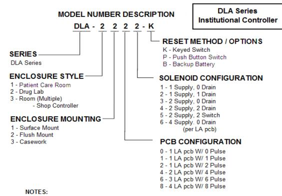
Style 1 is limited to 4 Solenoids W/ PCB Configuration 0, 1 & 2 only.
